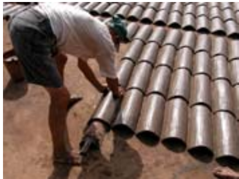
Trabajador laying out green tejas to dry in the Nicaraguan sun. Notice the curved paddle that is used to both form the tejas and carry it to the drying yard.
