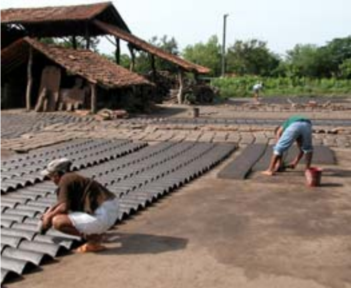
Green tejas being laid out to dry in the sun in the drying yard. Averaging drying time is two days. Tejas are in the foreground and bricks and floor tiles in the background.
