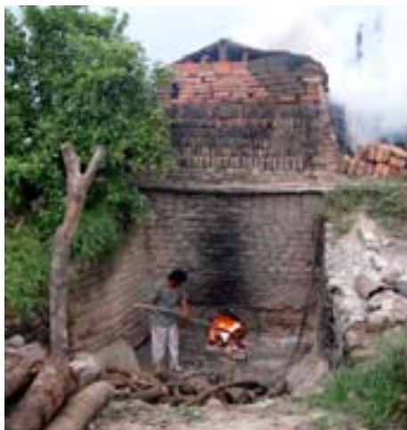
Bombero (fireman) loading wood into the kiln.
