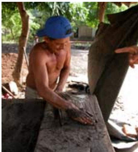
The tejas are made by hand by working the clay tightly into 9" x 16" x 1/2" wooden forms, which are then placed on a curved paddle to be carried to the drying yard.
